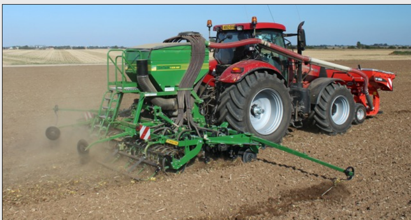
ADS seed metering and delivery. Hopper capacities range from 1000 litres to 3000 litres depending on the model.
