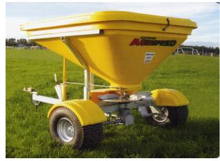
500 kgs Hopper capacity Spreading width 15m Height 1.40m Weight 375kgs Quad bike reg'd 4WD 400cc+
