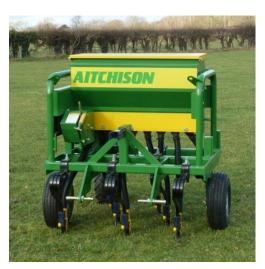
The **AITCHISON** Vineyard Drills offer the unbeatable 'inverted-T' sowing method, allied with the versatile and precise seed metering system, to those who wish to sow cover crops or even cash crops between rows of vines or trees. They may also be used for sowing conservation strips and field margins..
