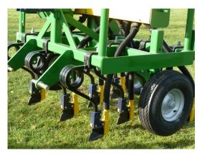
These small, simple drills are mounted behind a small tractor equipped with a hydraulic linkage, but may be adapted to be used behind quad bikes or 4wd picksups, etc.
